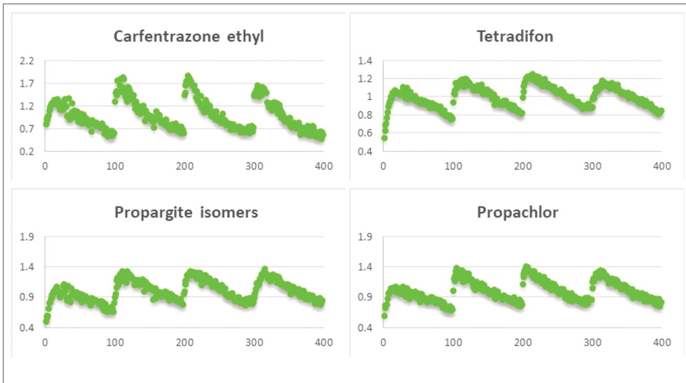
**Figure 3. Response trends of four different pesticides showing signal recovery after only inlet maintenance and guard column trimming.**
