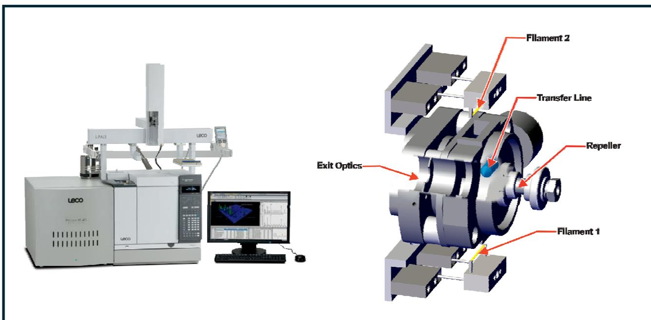
**Figure 1. The Pegasus BT 4D and a simplified drawing of the StayClean ion source. The source filaments can be quickly changed without source disassembly, while the overall source design ensures maximum system stability and minimizes maintenance downtime.**
