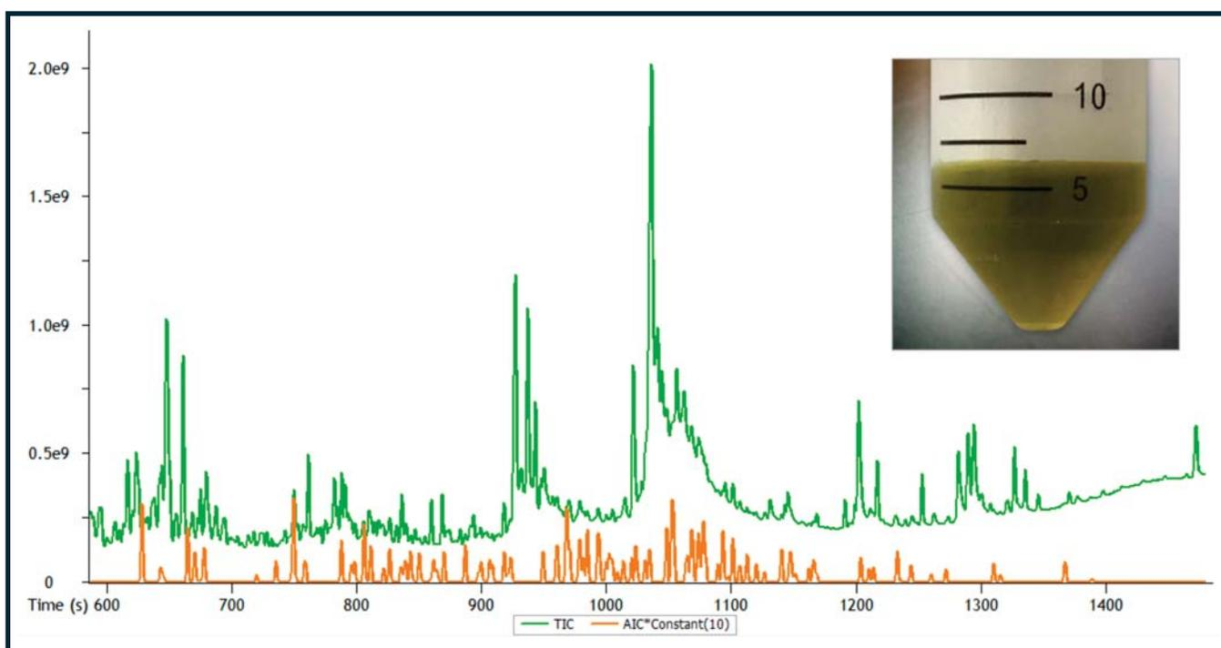
**Figure 2. Total Ion Chromatogram (TIC) of the spiked spinach extract and Analytical Ion Chromatogram (AIC). The AIC is filtered to display pesticide signals ONLY, and is multiplied by 10 for visualization purposes. The insert is an image of the QuEChERS spinach extract.**
