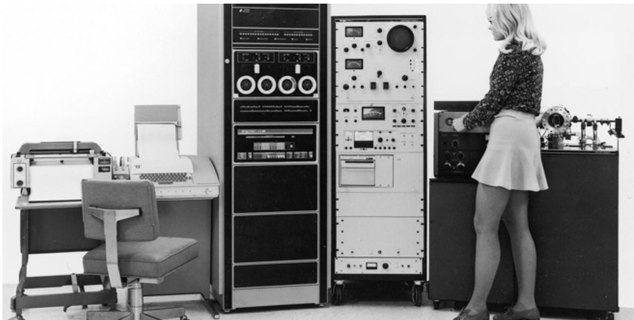
A Finnigan Instrument Corporation Model 1015 GC/MS/DS. From left to right: a minicomputer from Digital Equipment; part of the quadrupole mass spectrometer; the remainder of the mass spectrometer electronics console and gas chromatograph. Image courtesy of Robert Finnigan.
